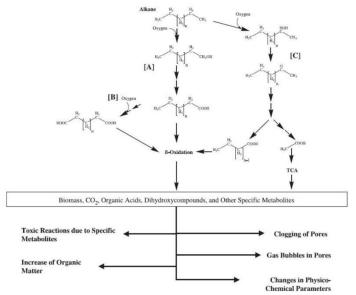
Figure 1 Aerobic biodegradation of n-alkanes (Hassanshahian and Capello, 2012)
